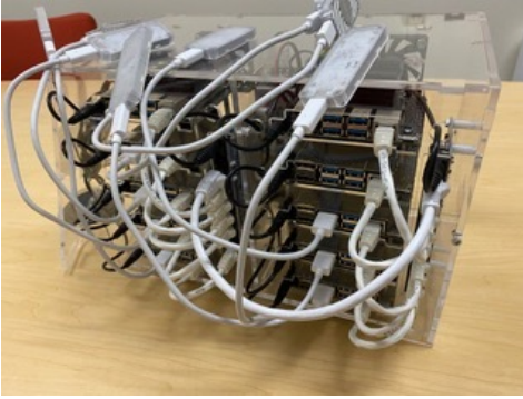
Fig. 14. 10-node Jetson Nano cluster
